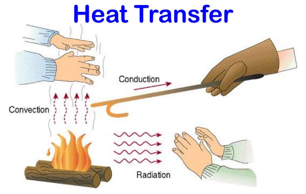
Conduction is by hot molecules colliding with neighbors Convection is by hot stuff moving in bulk from place to place
